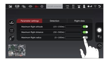
Click the " (icon to enter the setting interface (as shown in the figure above). This allows you to set a limited flight range:
